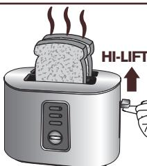
To remove smaller-sized breads after the toasting cycle.
