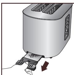
■ A removable crumb tray is provided for easy cleaning. Pull out the tray completely and discard the crumbs.
