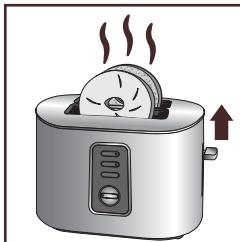
■ The toasting chamber automatically lifts once toasting cycle is complete.
