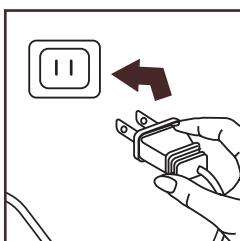
■ Unwind the power cord completely. Never operate with cord partially unrolled. Plug the toaster into the wall outlet.
