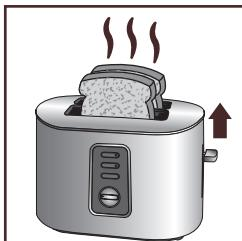
■ The toasting chamber automatically lifts the toast and lever once the toasting cycle is complete.
