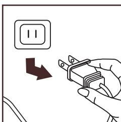
■ Unplug the toaster from the wall outlet and allow the toaster to cool completely, approximately 10 minutes.
