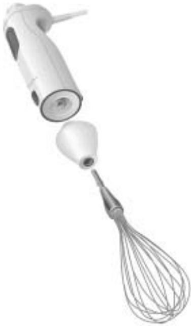
2. Insert the whisk adapter into the motor body. Adapter automatically adjusts the whisk to the proper range of speeds appropriate for whipping.
